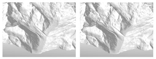
**Figure 1.** Visualisation of the created DEMs for the Bernina region in a block diagram (left: 1935, right: 2008) (Bruengger 2012)
