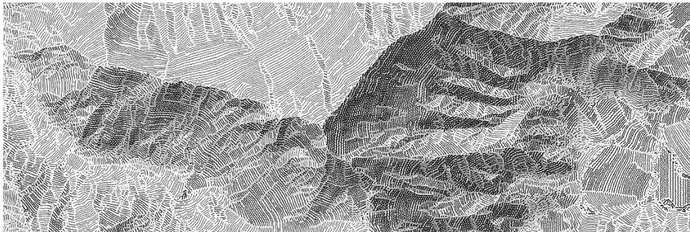
**Figure 17.** Automated rock drawing for the SWA Everest map. Generalized shaded relief to delineate morphological units combined with automated filling with light-modulated hachures. Note that areas without rock are not yet masked out!
